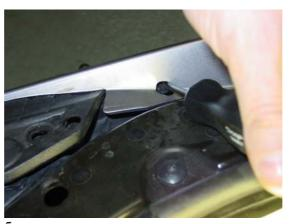
2/ Remove the front crash bar, this will require a 16mm socket and a spanner in order to release fully. Remove the 2 air deflectors either side of the intercooler, these are only clipped into place and can be simply moved to the side in order to gain access to the Intercooler hose connections. Now release the right and left hose clip connections and then the hoses to the intercooler. The intercooler can now be lifted up from its rear fixings and removed from the vehicle.
