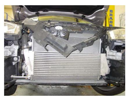
3/ Now fit the uprated intercooler in to place. Refit and tighten the 2 hose connections. You will now need to cut the plastic air diverters to suit the new intercooler shape; this can be done with a suitable sharp craft knife, hot knife or hacksaw. You can now refit the crash bar and complete bumper section in reversal of removal.
